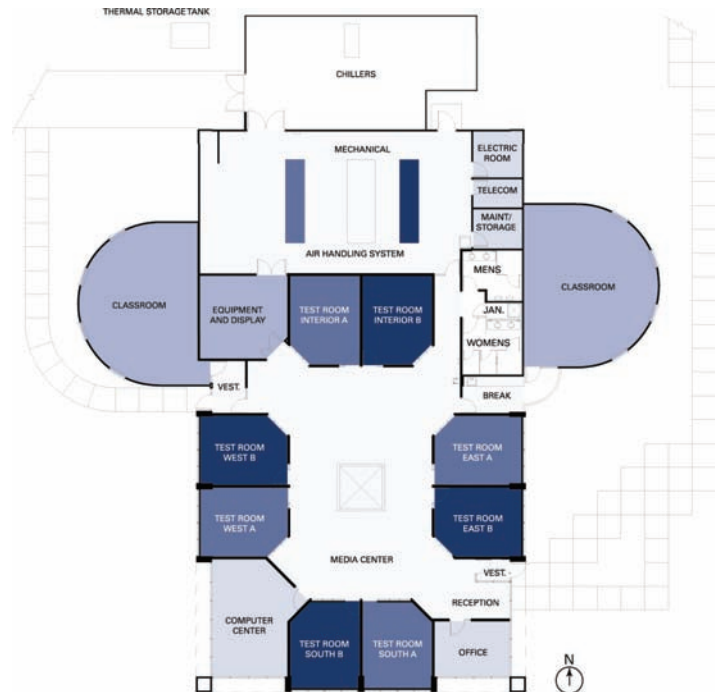
Figure 2-1: Schematic of the side-by-side test rooms of the Energy Resource Station.
