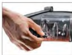
Continuous condensate drain-off for long term measurements
